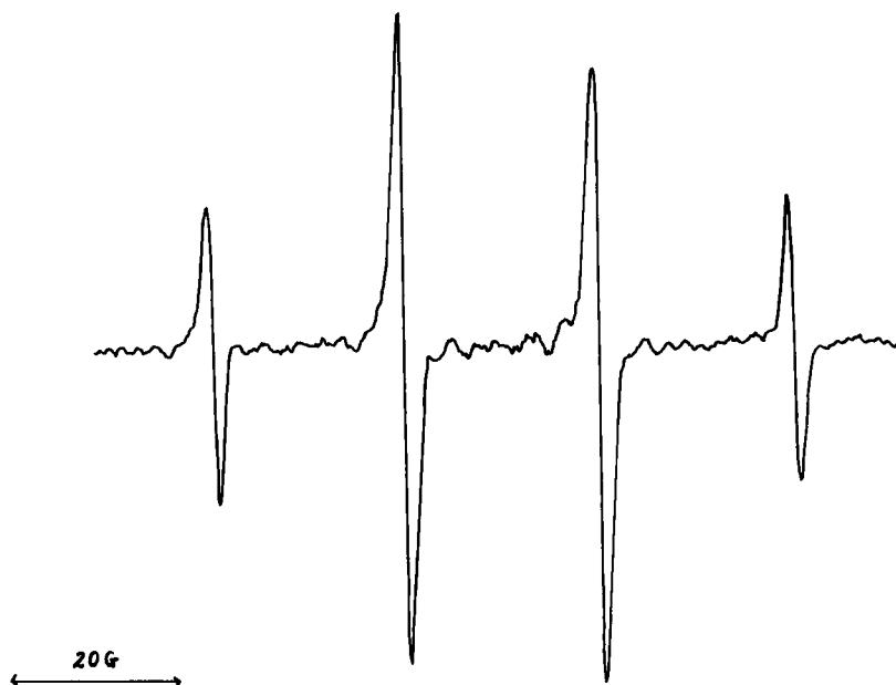
FIG. 2. ESR spectrum of the radical formed from diallylmalonic acid and amino radicals.
